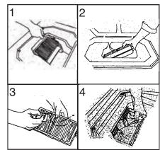
To clean the combustor, (1) remove the two bolts holding the catalyst in place. (2) Tilt the combustor to remove it from the stove. (3) Brush both sides of the combustor and (4) brush the baffle
